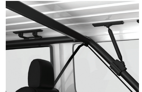
▶ The internal supports attach to the roll cage ensuring lateral stability for maximum strength.
