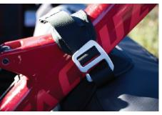
SitTight™ cradles with a new G-Hook tension lock system are easy on carbon bike frames and painted surfaces.
