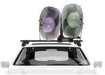
Capable of carrying two boats when set to stacker position (second set of straps and bow-stern tie downs required).
