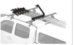
Clamshell open and close makes loading up rods easy and the protective padding protects rods.
