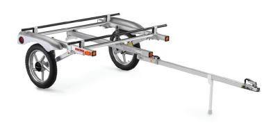
Made of lightweight aluminum, RACKandROLL carries gear easily upon shock absorbers that provide a full 4" of independent wheel travel.
