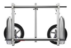
The wheels of the trailer are easily removable to make for easy upright storage in a small space.
