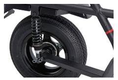
Shock absorbers allow for an easy ride for loaded-up gear.
