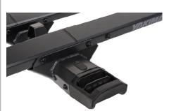
Ergonomic, forward facing remote tilt lever with action release tilts loaded rack forward.
