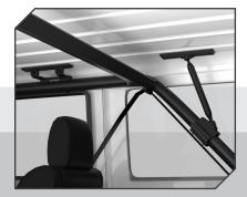
THE INTERNAL SUPPORTS ATTACH TO THE ROLL CAGE ENSURING LATERAL STABILITY FOR MAXIMUM STRENGTH.
