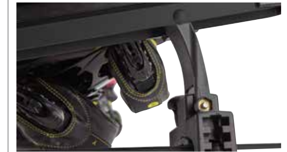
SkiLift attachment provides clearance for tall bindings.
