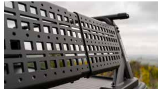
Allows for crossbar spreads from 40 to 54 inches.
